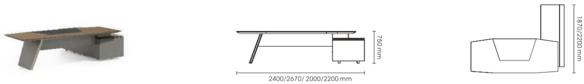
FGY80L.24/FGY80L.26/FGY80L.30 L2400\*W1870\*H750 / L2670\*W1870\*H750 / L2000\*W1670\*H750 / L2200\*W1670\*H750 (mm)
